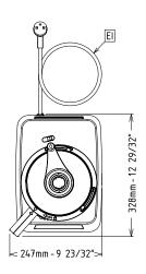
Electric Supply voltage: 220-240 V/1N ph/50/60 Hz Electrical power, max: 0.75 kW 0.75 kW **Total Watts:** Capacity: Performance (up to): Capacity: 2.6 litres Key Information: External dimensions, Width: 247 mm External dimensions, 328 mm Depth: External dimensions, Height: 456 mm 16.6 kg **Shipping weight:** Meat mincing capacity: 0 kg Mayonnaise preparation 0 kg capacity: Pastry preparation capacity:
